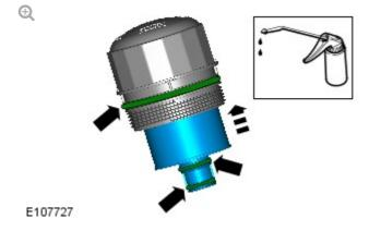
Lubricate the oil filter element O-ring seal with clean engine oil.
