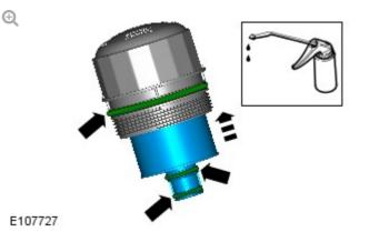
Lubricate the oil filter element O-ring seal with clean engine oil.
