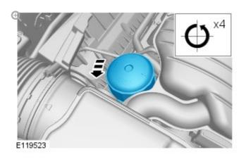
Allow the engine oil to drain from the oil filter element housing for two minutes.
