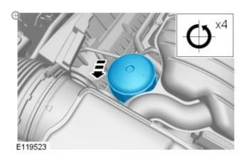
Loosen the element cover 4 complete turns to allow engine oil to drain from the filter cover.
