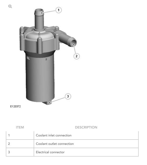
The charge air coolant pump is an electric pump attached to the LH (lefthand) side of the radiator pack frame. Hoses connect the inlet of the charge air coolant pump to the charge air radiator, and the outlet to the charge air coolers. An electrical connector provides the interface between the motor of the charge air coolant pump and the vehicle wiring.
