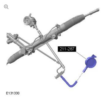
Connect the pressure gauge to the special tool valve block.
