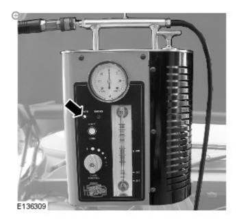
Observe the power indicator lamp on the smoke test equipment. Make sure that a continuous green light is displayed.
