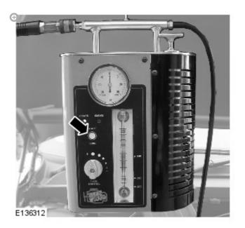
Switch the smoke test equipment on.
