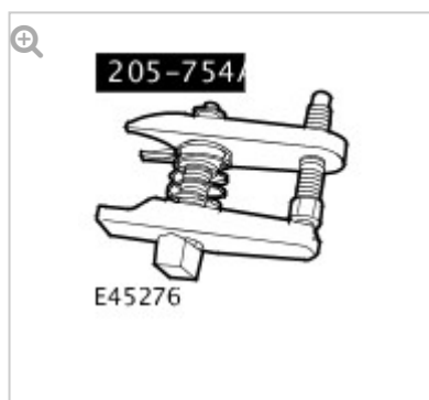
205- 754(LRT- 54-027) Ball joint separator
